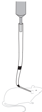
Attach a 1.2Fr catheter directly to a 22 or 25ga swivel
